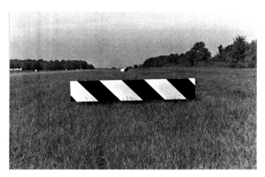
FIGURE 4. AIMING POINT MARKER
