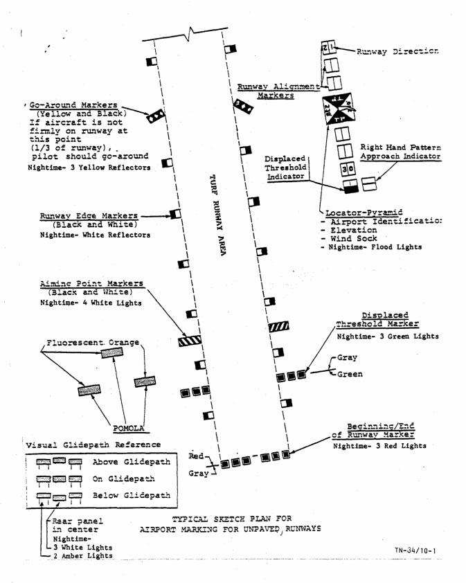
FIGURE 1. TYPICAL SKETCH PLAN FOR AIRPORT MARKING FOR UNPAVED RUNWAYS
