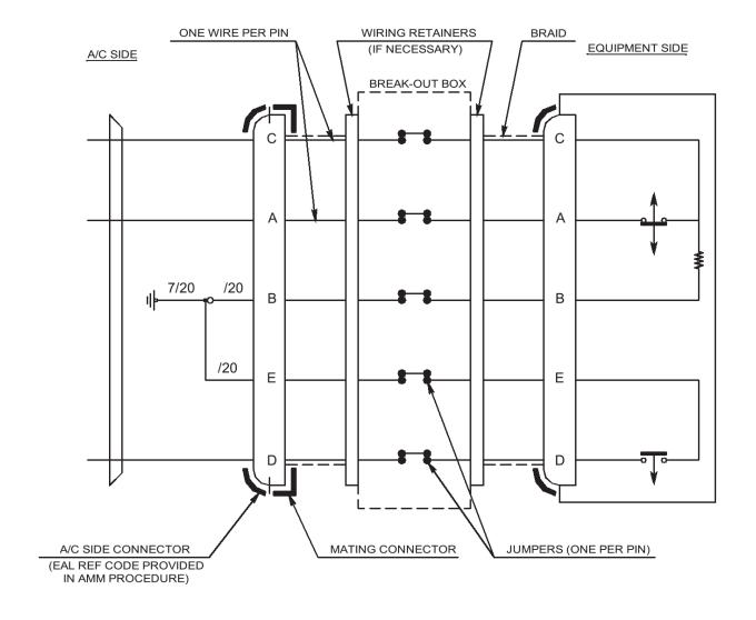
Figure 1: BREAK-OUT BOX DESIGN DRAWING
